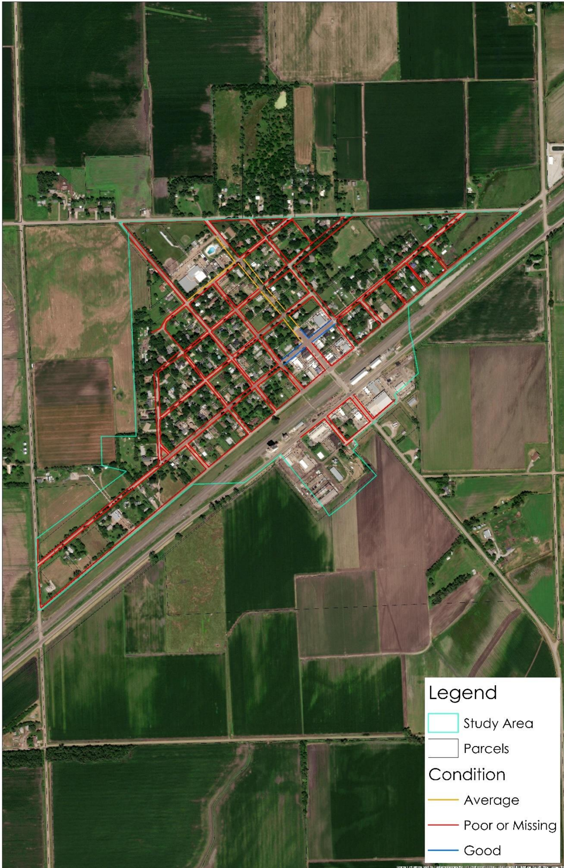
Figure 6 Curb and Gutter Conditions
